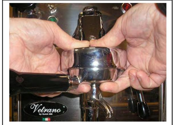
Maintenance Tip: Replacing the gasket on a yearly basis will make the replacement procedure much easier. There are also benefits to having a new gasket. It will provide a better seal for a better espresso extraction and it also enables you to be able to remove the shower screen without ruining the gasket to provide for better cleaning which will result in better tasting shots.
